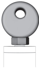
Correct installation of PATROLMED on TOWER - TOWER22 - TOWERA2 support
