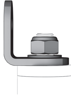
Correct installation of PATROLTERM on TOWER - TOWER22 - TOWERA2 support
