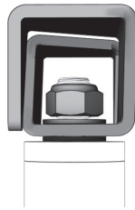
Correct installation of PATROLINT on TOWER - TOWER22 - TOWERA2 support
